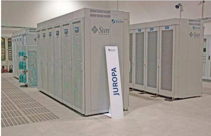
Figure 1.3: Cabinet of parallelised Intel dual-core processors, part of the JUROPA supercomputer at Jülich Supercomputing center.
